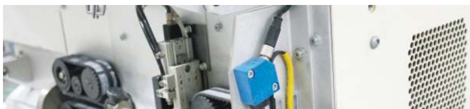
连接线缆及分线盒 Connection cables & Distribution Box
